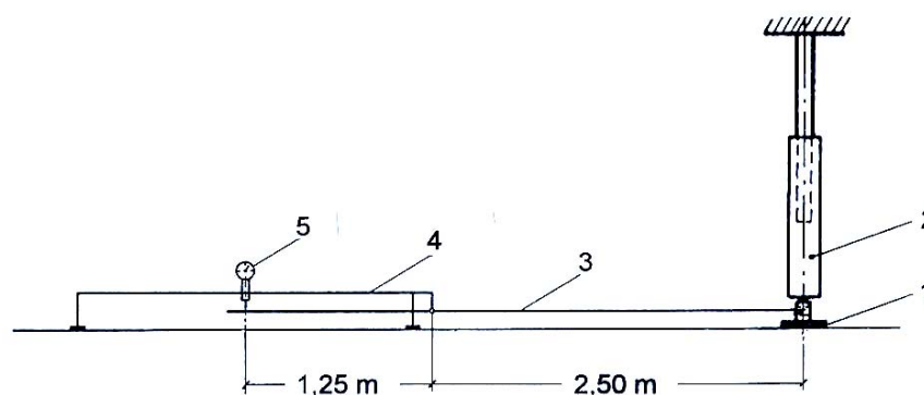
Fig. 2: Scheme of settlement measurements using single measuring gauge (with Benkelman beam)
