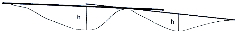
Fig. 1: Placing straight edge to assess deviation of individual unevenness h on pavement surface
