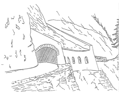
Figure 6.34: A gallery protects the road against falling rocks and snow avalanches
