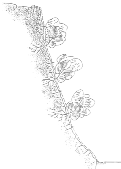
Figure 3.36: Protection of friable slope by rockfall netting - drapes. Introduced vegetation is developing into base (M. Plešnar)
