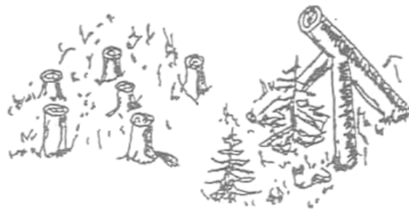
Figure 6.29: Vegetation protection against the consequences of sliding, slipping and gliding of snow by simple supporting structures, which increase the roughness of the surface.
