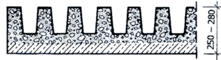
Figure 6.5: Cross section of high absorption noise protection element made from light material
