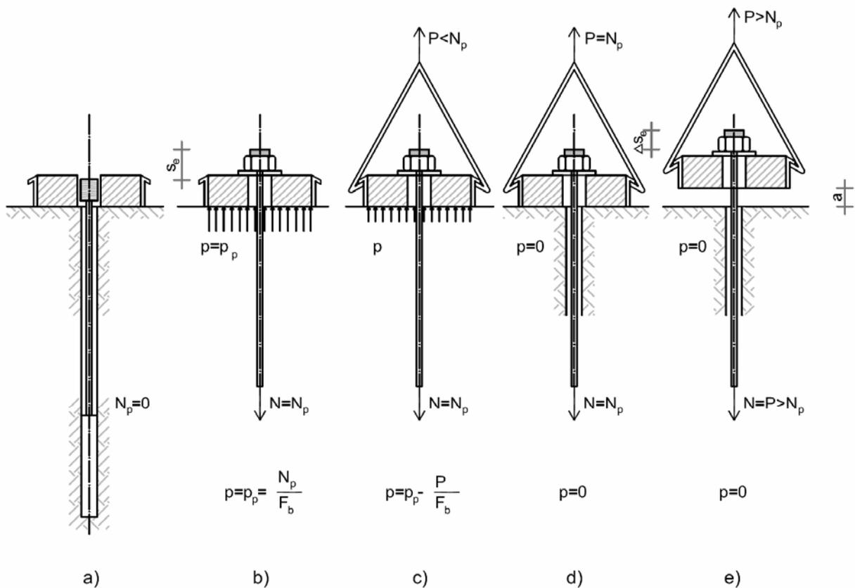
Fig. 9.2: Scheme of functioning of pre-stressed ground anchor
