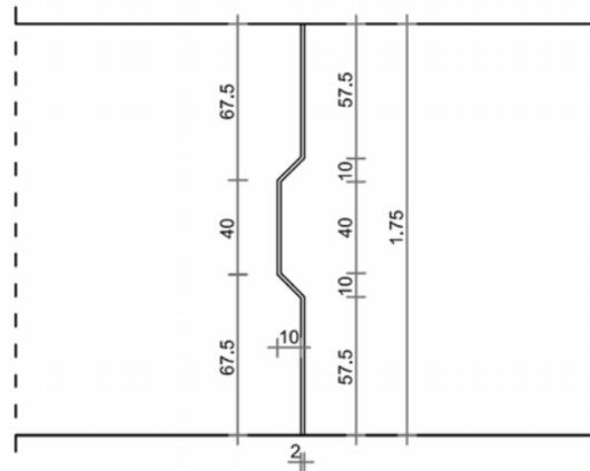
Fig. 5.19: Linking beam expansion joint in plan
