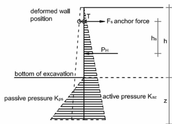
Fig. 6.3: Pressure distribution and displacements for a pile wall, anchored at one level
