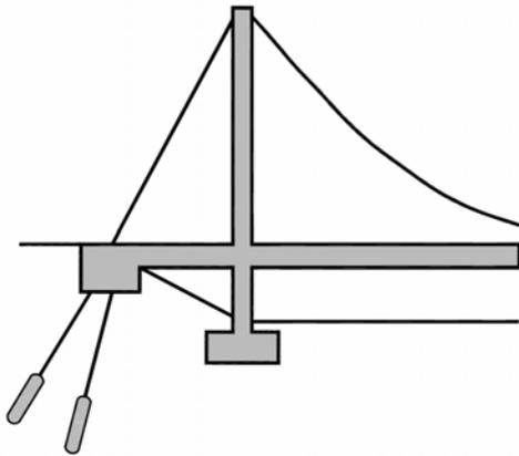
Fig. 9.8: Anchor block of cable-stayed bridge
