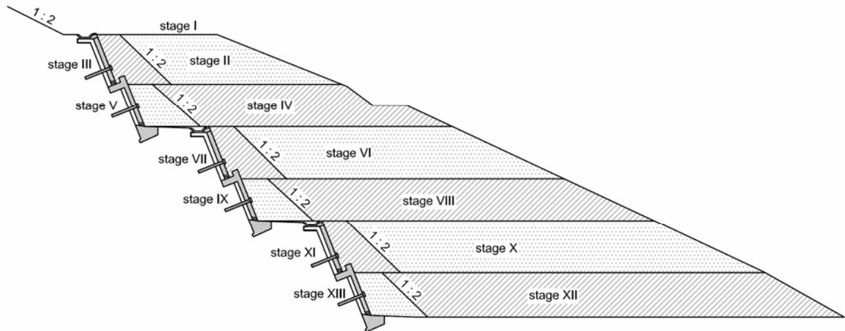
Stage I: Wide excavation by the road contractor up to linking beam
