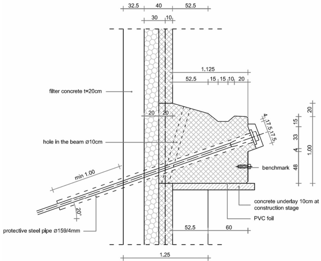
Fig. 5.17: Cross section of intermediate anchor beam
