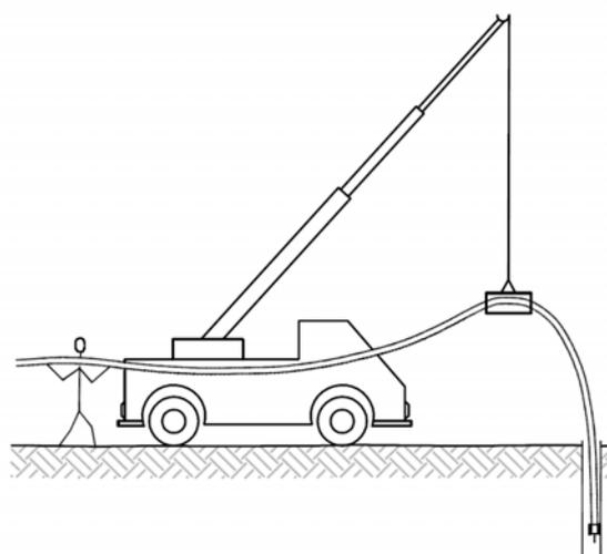
Fig. 9.5: Installation of anchors by means of a mobile crane
