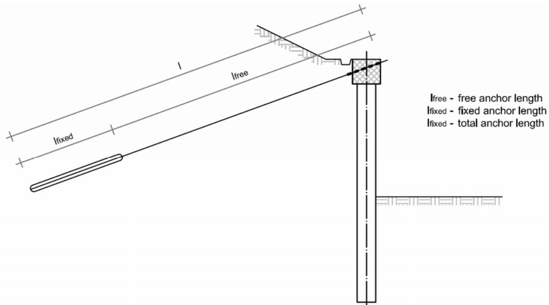
Fig. 4.11: Pile wall with anchors on top
