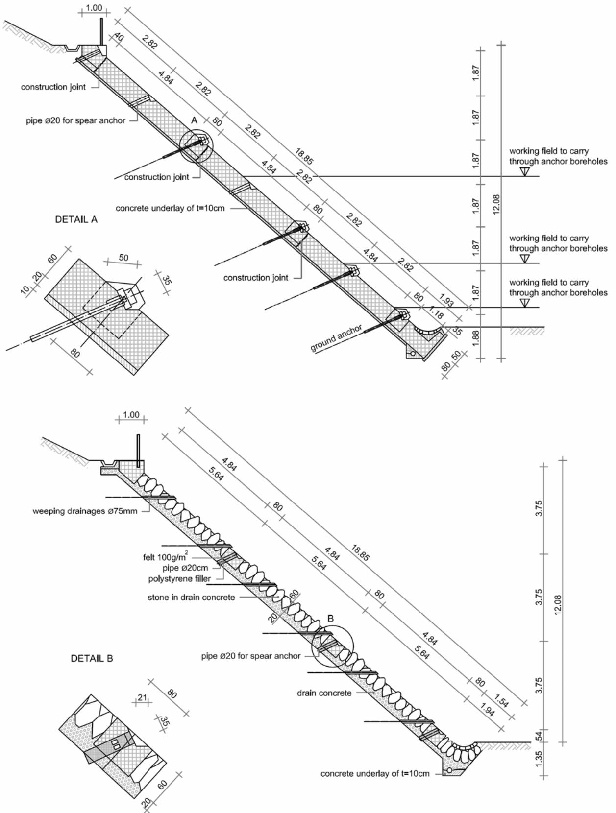
Fig. 5.9: Anchor columns and beams – grid structure with filling elements in-between
