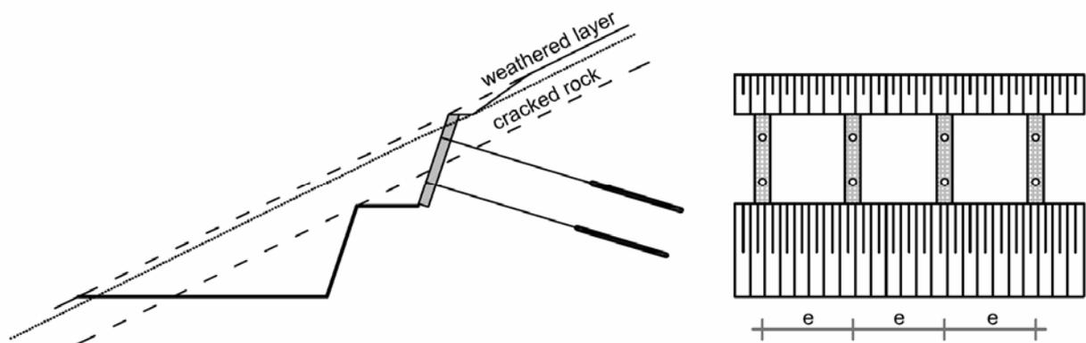
Fig. 4.2: Anchored columns
