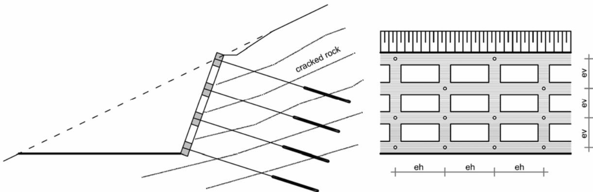
Fig. 4.5: Anchored columns and beams – grid structure
