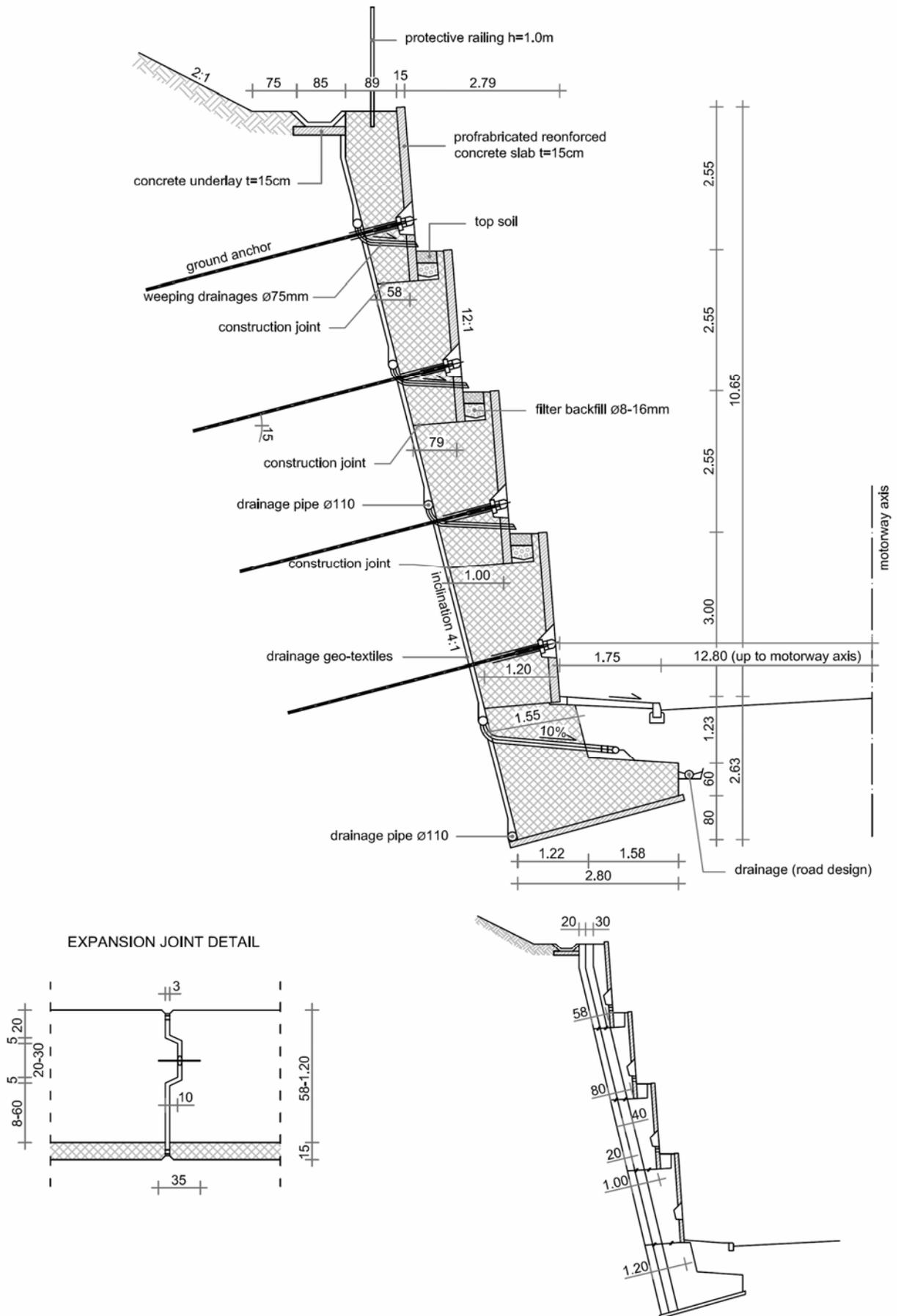
Fig. 5.13: Characteristic cross section of an anchored wall constructed from above downwards
