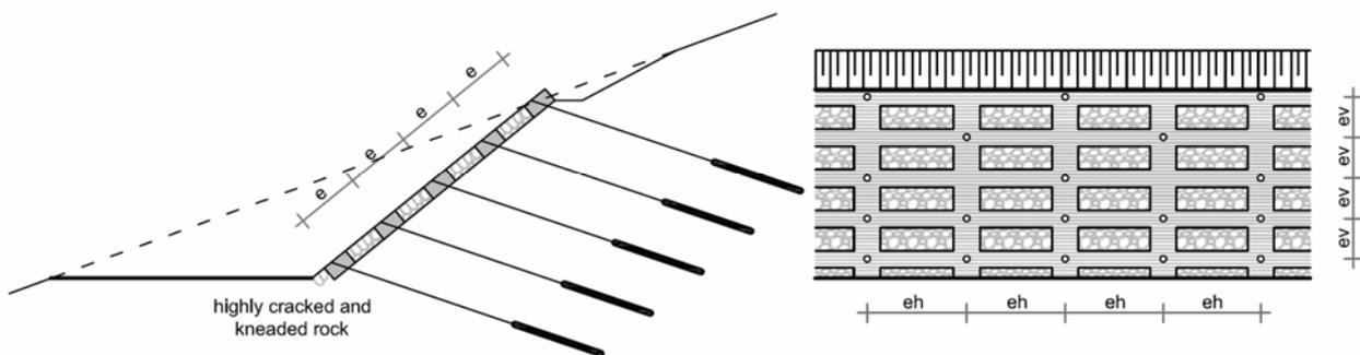
Fig. 4.6: Anchored columns and beams – grid structure with filling elements in-between
