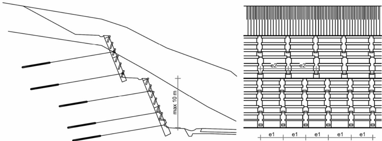
Fig. 4.3: Anchored columns with filling elements in-between
