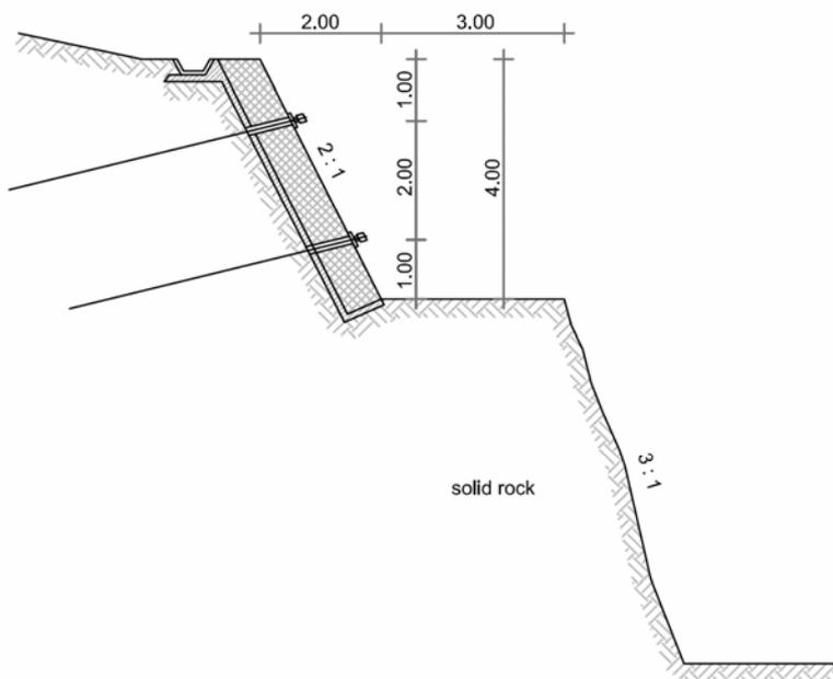
Fig. 5.4: Anchored columns
