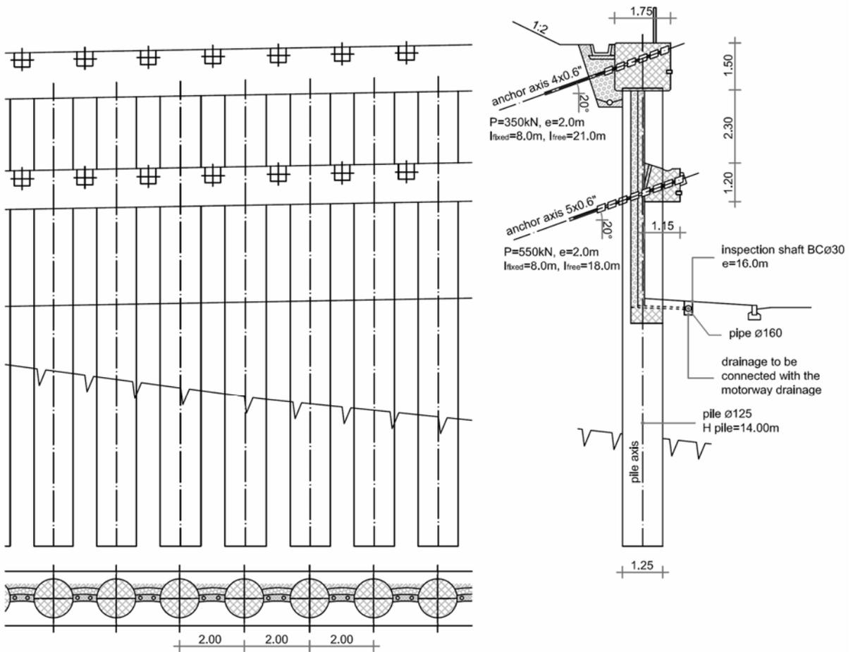
Fig. 5.14: A portion of a pile wall anchored at two levels
