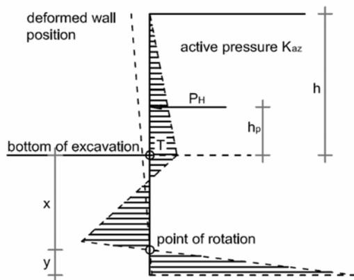
Fig. 6.2: Pressure distribution and displacements for a cantilevered pile wall
