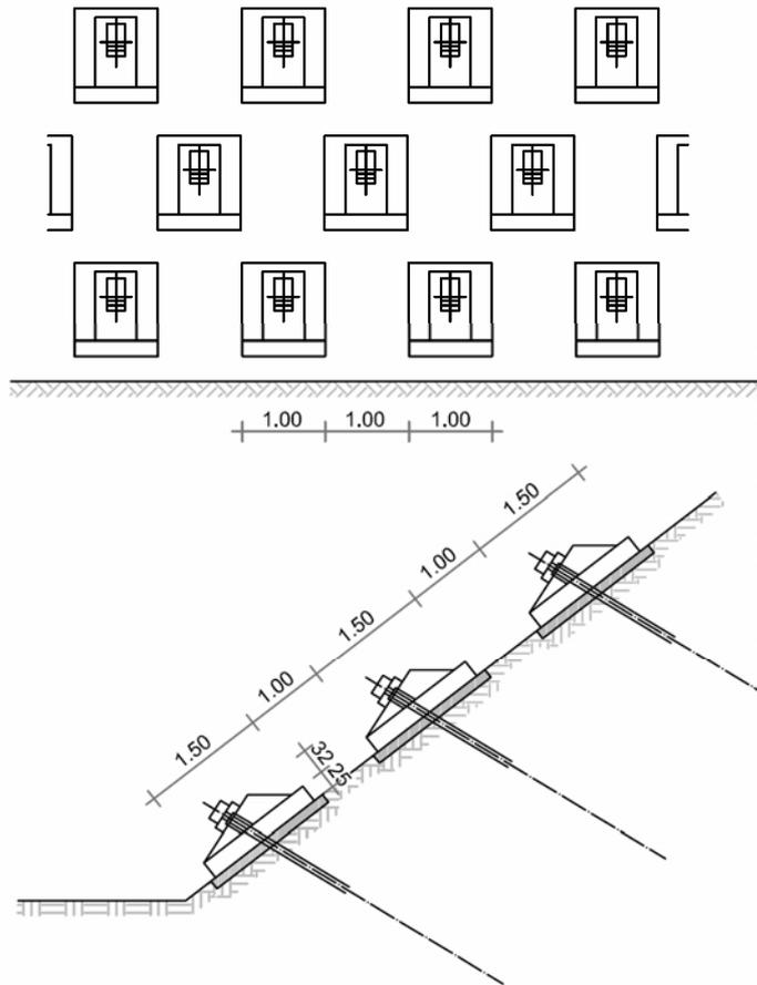
Fig. 5.2: Three-sided prismatic anchored block
