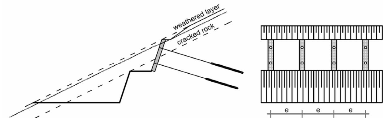
Fig. 4.2: Anchored columns
