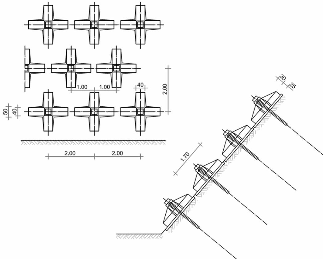
Fig. 5.3: Starry anchored block
