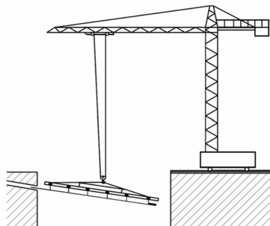
Fig. 9.4: Installation of anchors by means of cranes
