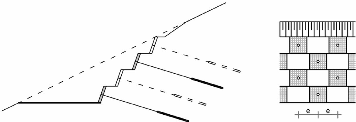
Fig. 4.1: Anchored blocks
