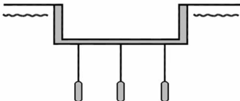
Fig. 9.9: Anchoring to take forces due to water buoyancy
