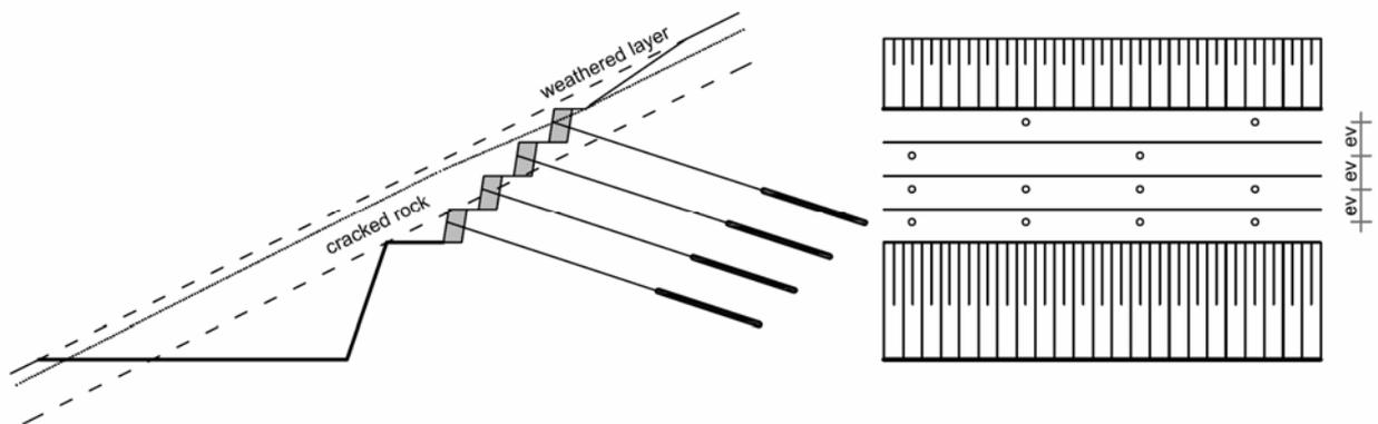
Fig. 4.4: Anchored beams
