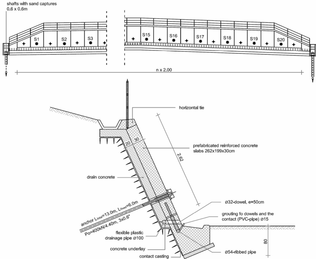
Fig. 5.12: Partly prefabricated anchored wall
