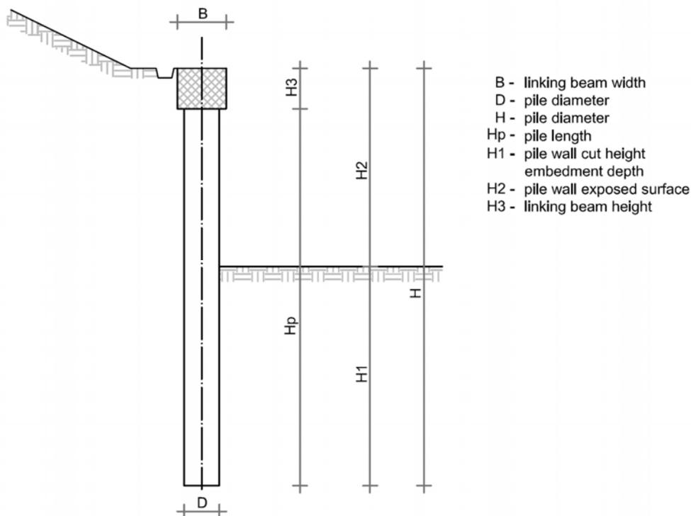
Fig. 4.10: Pile wall without anchors
