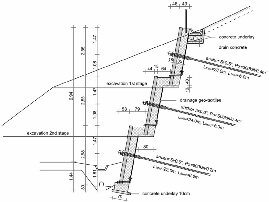
Fig. 5.11: Semi-prefabricated anchored wall
