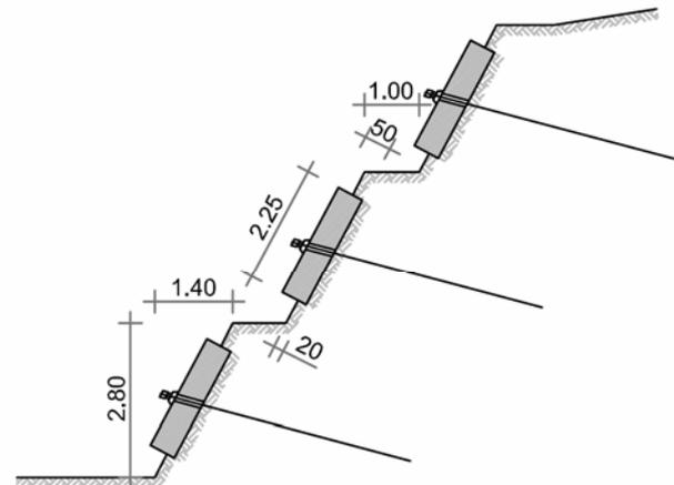
Fig. 5.1: Rectangular anchored block
