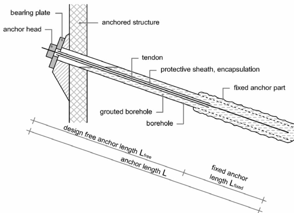
Fig. 9.1: Pre-stressed ground anchor with typical elements and symbols
