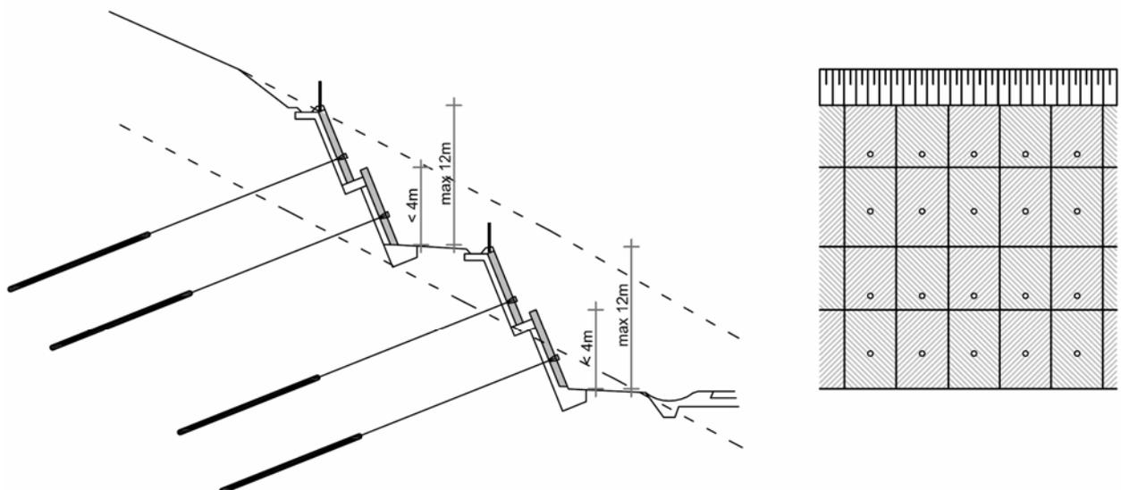
Fig. 4.8: Anchored wall composed of several segments
