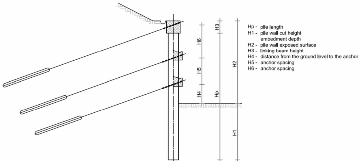
Fig. 4.12: Multiple-anchored pile wall
