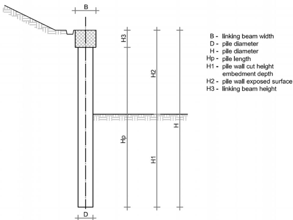
Fig. 4.10: Pile wall without anchors
