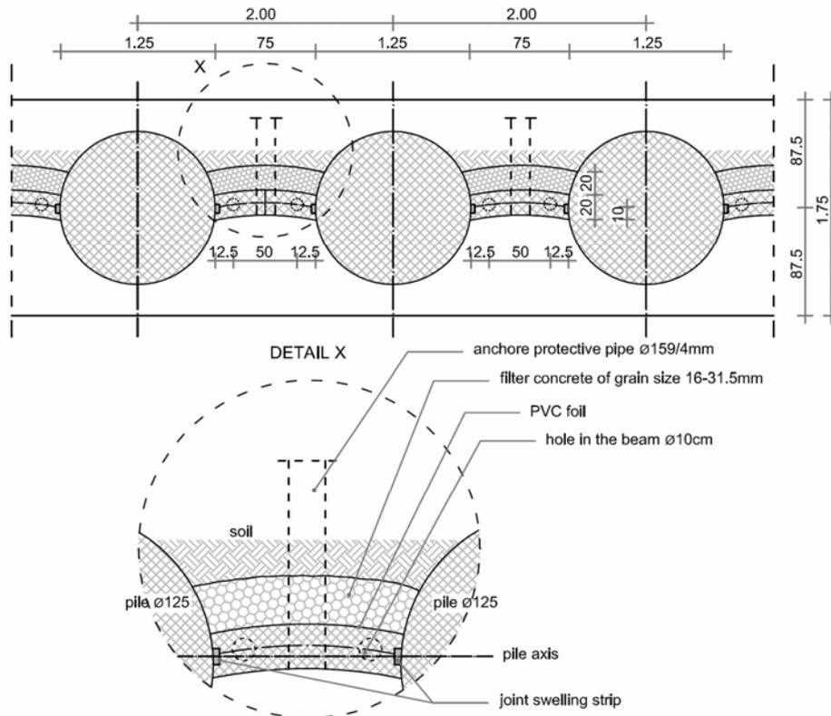
Fig. 5.15: Fillers between piles
