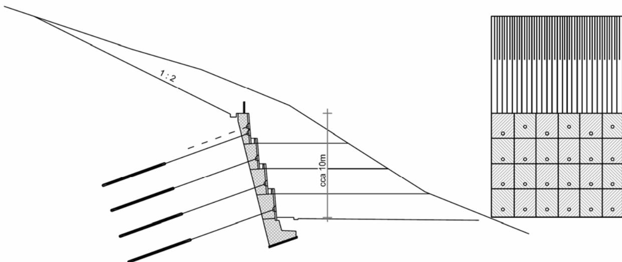
Fig. 4.9: Anchored wall constructed from above downwards
