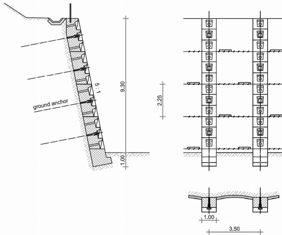
Fig. 5.5: Anchored columns with shot cement concrete in-between
