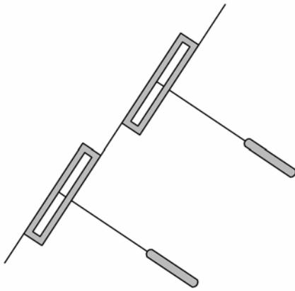
Fig. 9.7: Anchored blocks on rocky slope
