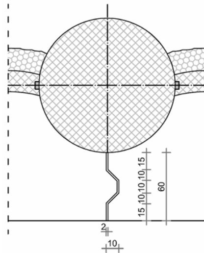
Fig. 5.20: Intermediate anchor beam expansion joint in plan
