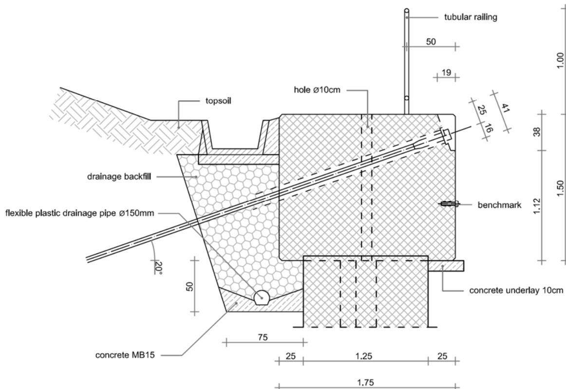
Fig. 5.16: Cross section of linking beam
