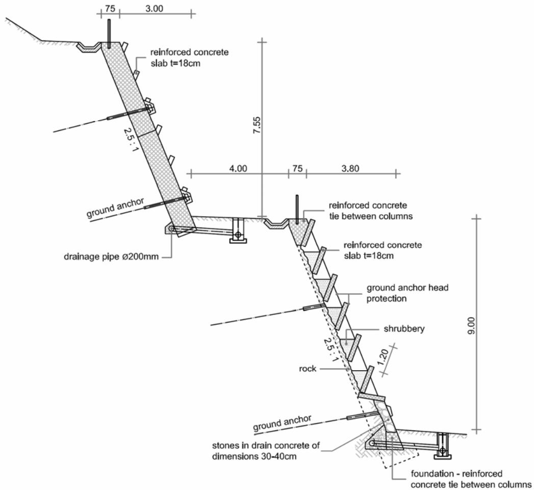
Fig. 5.6: Anchored columns with reinforced concrete slabs in-between
