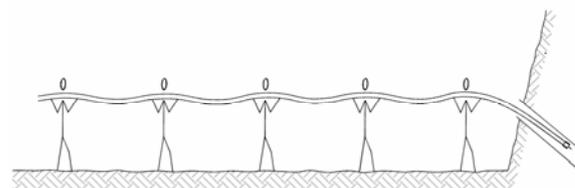
Fig. 9.3: Manual installation of anchors
