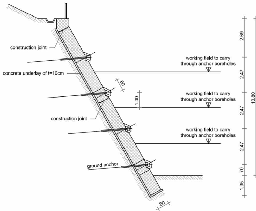
Fig. 5.8: Anchored columns and beams – grid structure
