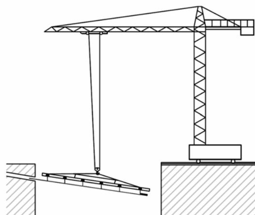
Fig. 9.4: Installation of anchors by means of cranes
