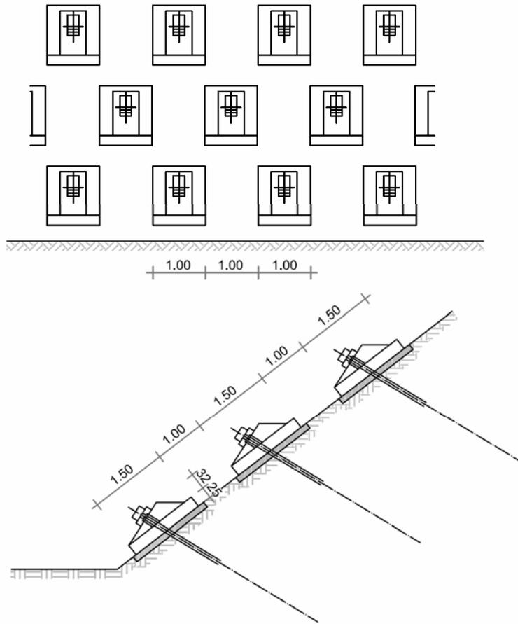
Fig. 5.2: Three-sided prismatic anchored block
