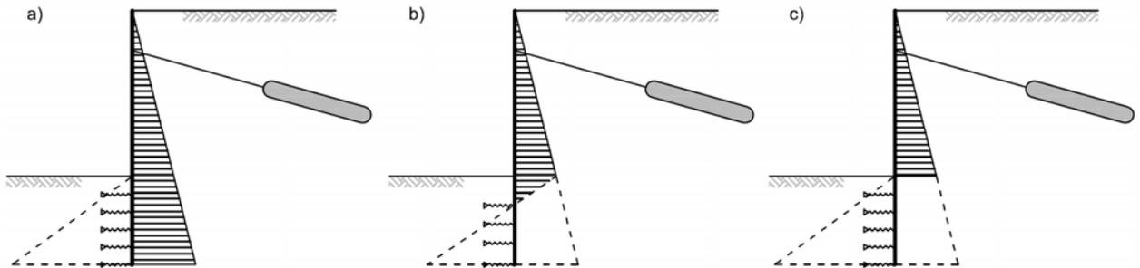
Fig. 6.1: Possible calculation methods in the static analysis of a pile wall, anchored at one level, using the modulus of reaction of the ground
