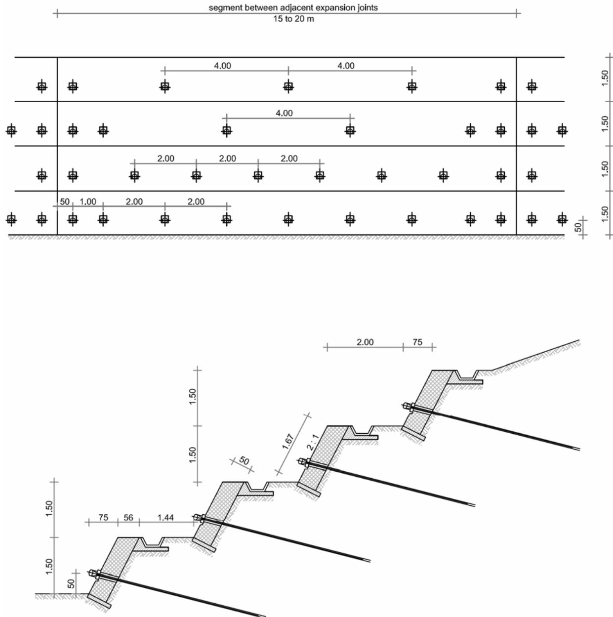
Fig. 5.7: Anchored beams
