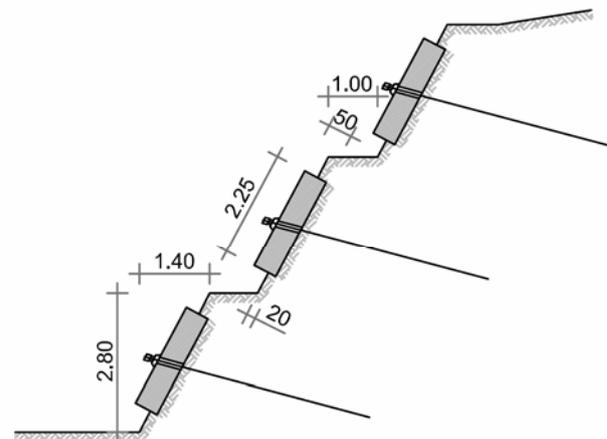
Fig. 5.1: Rectangular anchored block
