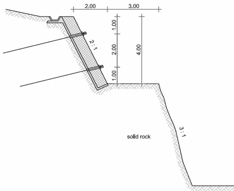
Fig. 5.4: Anchored columns
