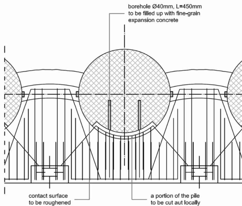
Fig. 5.18: Connection of intermediate anchor beam with piles
