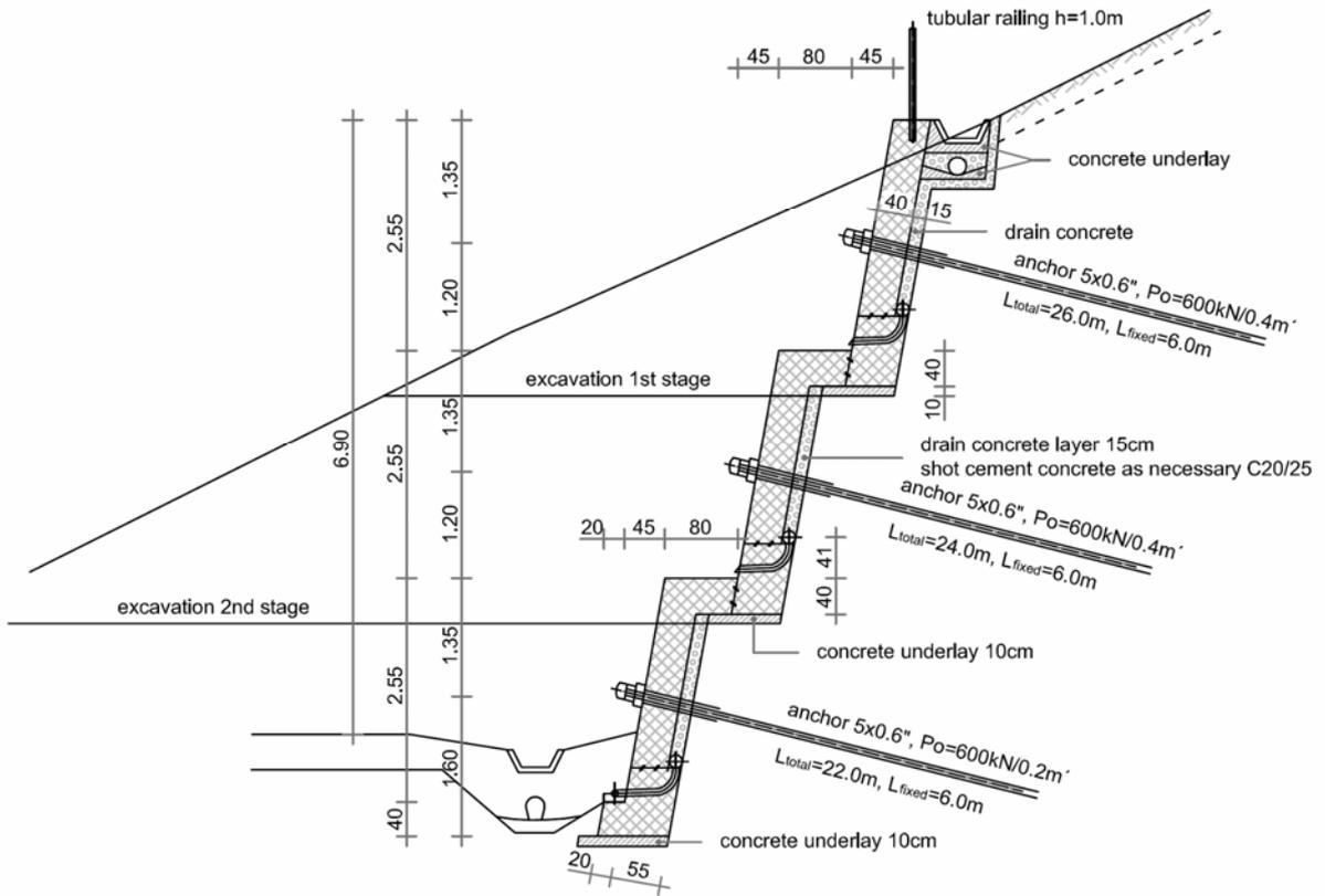
Fig. 5.10: Cast-in-situ anchored wall
