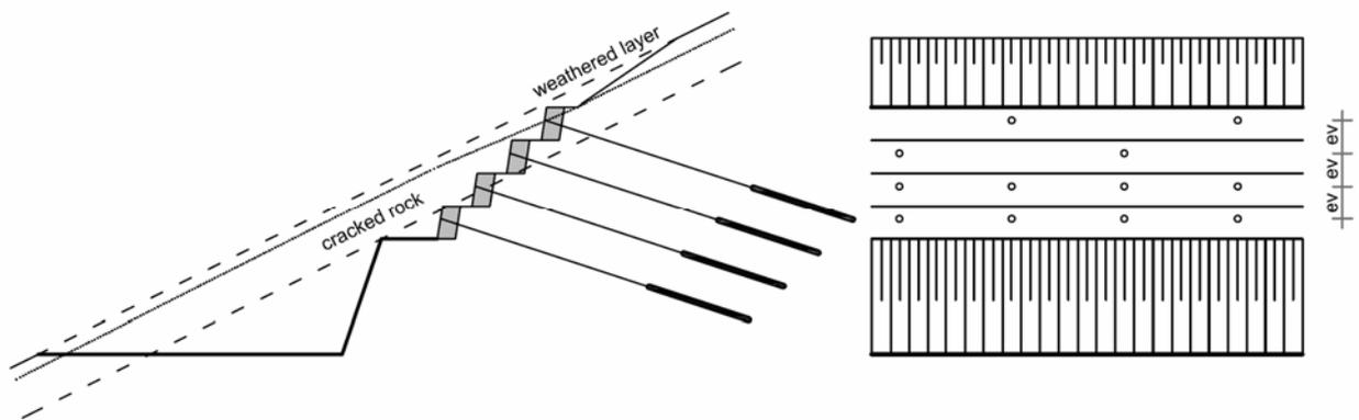
Fig. 4.4: Anchored beams
