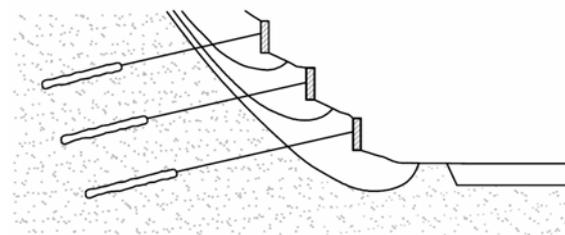
Fig. 9.6: Retaining structure anchors
