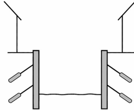
Fig. 9.10: Anchoring of construction pit protective walls
